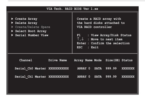
On the upper-right side of the screen is the message and legend box. The keys on the legend box allows you to navigate through the setup menu options. The message describes the function of each menu item. The following lists the keys found in the legend box with their corresponding functions.
